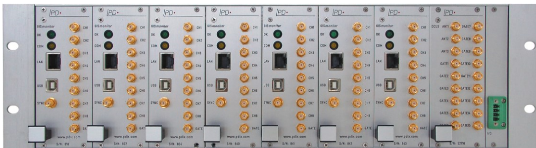
Fig. 7: GISmonitor acquisition frame with seven plugin boards
