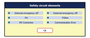
In order to close the dialog and proceed with the actual measuring operation, all signaled problems must first be solved. The status of the respective elements can be read from the color of the status icon:
