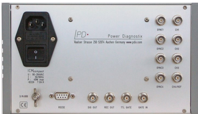
Fig. III.60: Back panel with MUX4 and RIV input
