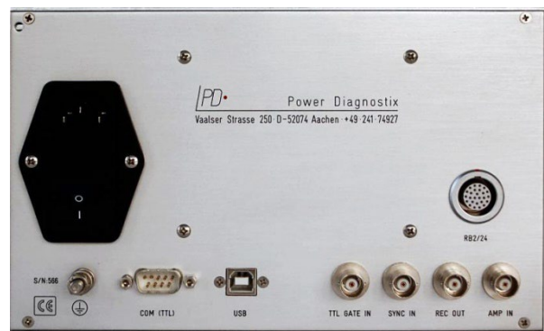
Fig. III.61: Back panel with MUX12 and TTL gating input
