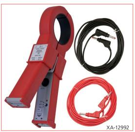
Dual Ground kit, XA-12990(max 200A), XA-12992(max 1000A) Max conductor size 50mm diameter(2"). Test cables 5m. Note: XA-12992 included in ordering art no. BB-59093
