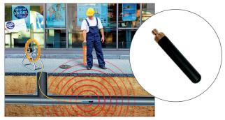
The MLS 55-3 pipeline transmitter probe is a slim, battery powered mini-transmitter and has a range of 5 m. When attached to a drain rod or fibreglass push rod cable by one of the 3 adapters provided, it is used to locate ductworks or blockages. A heavy duty protective cover is available.
