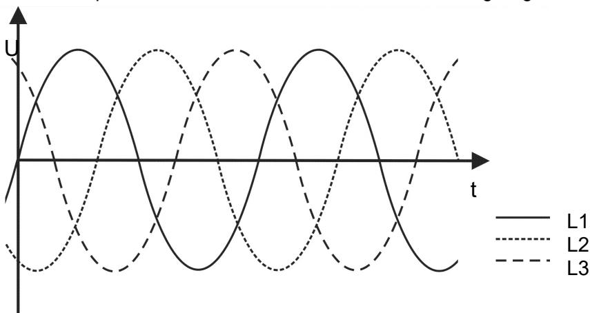
If we observe the phase shift ( $120^\circ$ ) of each alternating current curve in a vector diagram, the vectors form a symmetrical star:
