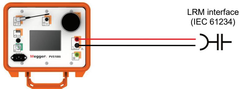
In combination with the „HR->LRM“ adapter it is also allowed to be connected to interfaces according to [IEC 61243-5 Type HR](#).
