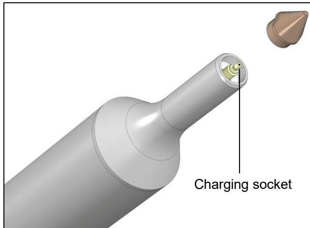
The charging procedure starts automatically ("Charge" LED lights up on the battery charger) and takes about three hours. After charging is completed, the battery charger switches to trickle charging ("Ready" LED is lit).
