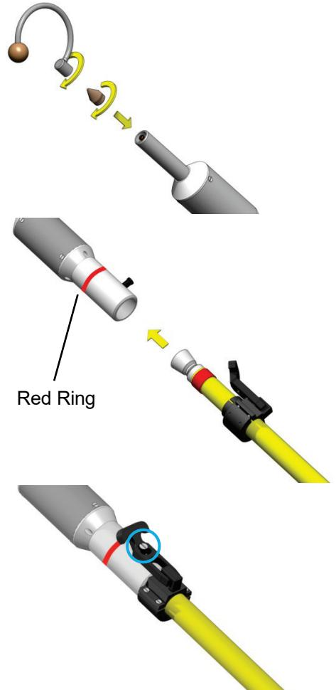
To create a contact between the contact pin of the sensor and the hot stick, push the hot stick into the base of the sensor until it reaches the stop.
