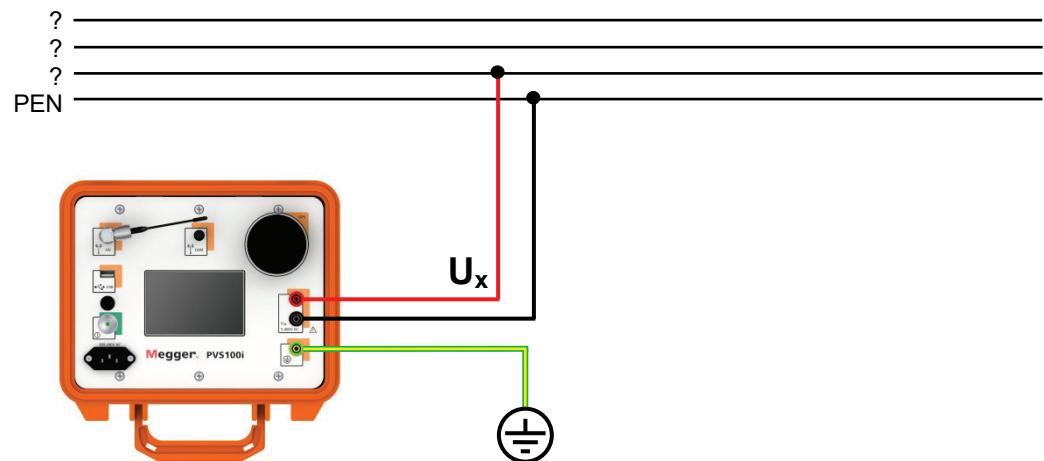
Direct tapping of LV HRC fuses Using the measuring cable MK 55 (available as a special accessory - see section 3.3) the test voltage can be directly tapped from LV HRC fuses of size 00 – 3 (6 ... 630 A).
