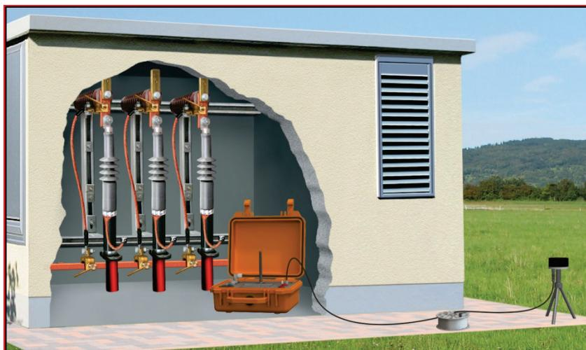
To do so, the GPS antenna must be removed from the base station (as shown in the following image) and screwed onto the stand. Once the stand is positioned on a clear surface outside of the building, the cable must be connected to the respective connectors on the base station and on the underside of the GPS antenna.
