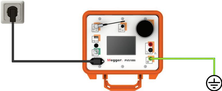
This supply voltage is normally also used as a reference voltage. If it is not suitable for some reason, the reference voltage can also be tapped from input  $U_x$  ⑨. The voltage supply from the mains supply must however also be ensured in this case!
