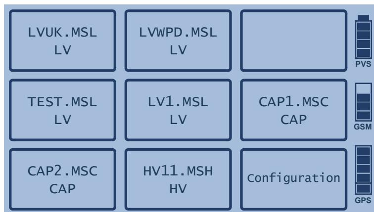
If the GPS power reserve is not yet sufficiently charged or the GSM reception quality does not provide reliable communication with the base (no bars or 1 bar), the individual measurement profiles cannot be selected and, accordingly, the measurement cannot be started.
