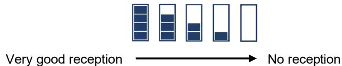
Under difficult conditions, e.g. within buildings, it may help to unscrew the rod antenna ⑥ and connect the external antenna (optional accessories) in its place. This should then be positioned outside the building if possible, or near windows.
