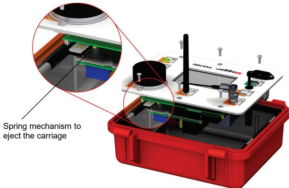
Briefly press on the yellow spring mechanism to eject the carriage from its position. The SIM card must then be inserted into the carriage and pushed into the guide until you feel a click.
