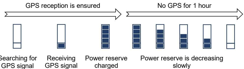
As illustrated by the above graphic, the internal power reserve synchronizes to the GPS signal as soon as it is received. Once this process is complete, a sufficiently accurate time base can be ensured even without GPS reception for an hour.
