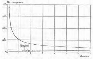
Fig. 8.—Leakage current plus charging current flowing into a rubber cable, from oup to 7 minutes.
