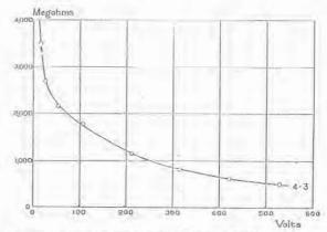
Fig. 15.—Insulation resistance of Paper; the same test-piece as in Fig. 14, but tested at o'l lb. per sq. inch.
