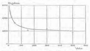
Fig. 28.—Characteristic curve obtained from a capillary glass tube filled with drops of water and bubbles of air, and arranged as shown in Fig. 27.
