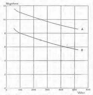
Fig. 7.—Insulation resistance of Interior Wiring, showing polarity, or "valve," effect (Ohmmeter test).
