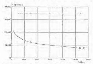
F16. 24.—Insulation resistance of varnished Cotton: (A) 12 hours and (B) 9 days after baking. Showing the change from Ohm's law (when the test-piece was dry) to moisture conduction after a few days' exposure to the air.
