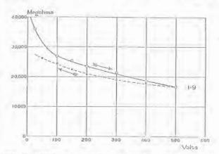
Fig. 5.—Insulation resistance of a moving-coil Ammeter in which the ebonile insulation had become defective from an accumulation of dirt.
