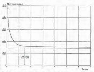
Fig. 9.—Leakage current plus charging current flowing into a rubber cable: continuation of the time-current curve in Fig. 8, ap to 7 hours.
