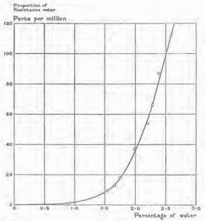
Fig. 26.—Proportion of resistance water to the total quantity of water in a pad of paper (see Table 1).
