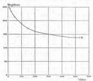
Fig. 18.—Insulation resistance of Micanile Cloth which contained moisture absorbed from the air.
