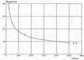
Pig. (2.—Insulation resistance of Cotton; continuation of the curve in Fig. 11 up to 500 volts.
