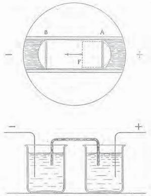
Fig. 27.—Elementary Model of an absorbent insulator. The upper figure represents one of the air bubbles as seen in the field of a microscope.
