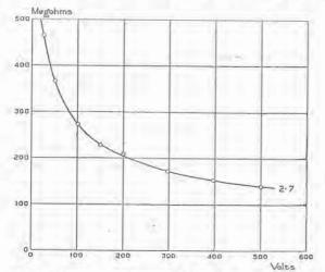
Fig. 13.—Insulation resistance of Cotlon; the same test-piece as in Figs. 10, 11, and 12, after further baking.
