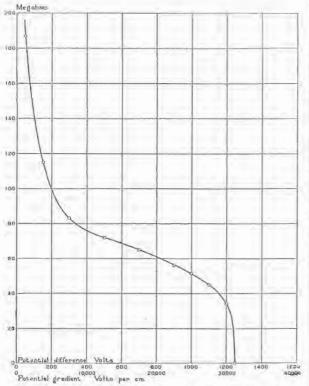
Fig. (.—Complete characteristic curve for Cotton containing a normal amount of moisture absorbed from the air.
