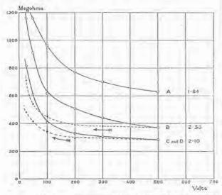
Fig. 29.—Characteristic curves obtained from a Model Insulator composed of 13 capillary glass tubes arranged in parallel.
