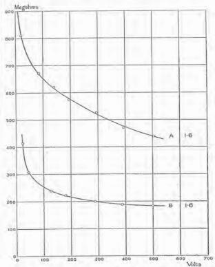
Fig. 3.—Insulation resistance of Field Coils: A, in dry weather; B, on a damp day.
