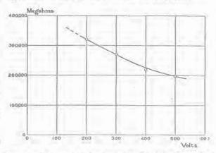
Ftg. 19.—The same test-piece as in Fig. 18 tested 24 hours after being dried in an oven. Note: One hour after removal from the oven this test-piece had a resistance of 1,300,000 megohms at 500 volts.
