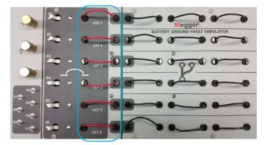
14. Notice that circuit 3 contains both the capacitive phantom fault as well as a resistive fault. You can use the bridge one the secondary side of the circuit to find where the capacitive phantom fault is and where the resistive real fault is.c
