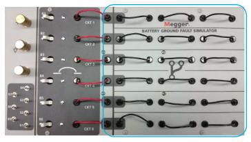
**NOTE:** This is one of the most difficult faults to locate because the impedance of the capacitance of the circuit is lower than the impedance of the fault.
