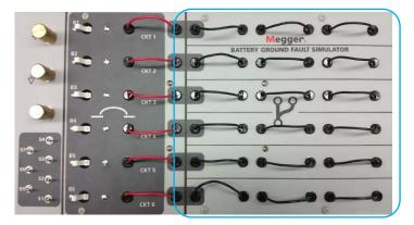
Results for Test #2 Switch S2 ON Circuit Characterization Capacitance =  $0\mu$ F (Minimal capacitance) Resistance = Less than 1K (Actually  $50\Omega$ ) Faulty Circuit = 2 Location of Short = Between loop 1 and 2
