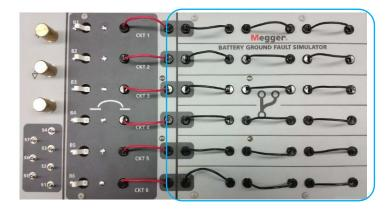
Results for Test #1 Switch S1 ON Circuit Characterization Capacitance =  $0\mu$ F (Minimal capacitance) Resistance = Approximately 2K Faulty Circuit = 1 Location of Short = Between loop 2 and 3
