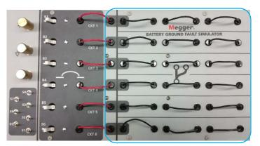
Results for Test #5 Switch S5 ON Circuit Characterization Capacitance = 0µF (Minimal capacitance) Resistance = Approximately >300K Faulty Circuit = 5 Location of Short = Between loop 1 and 2
