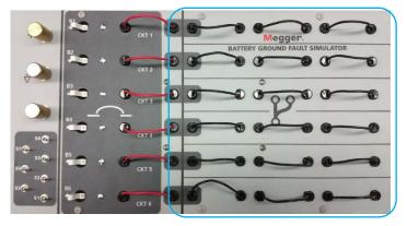
15. Once the first fault is found, remove it by opening the breaker. (This is only for training purposes. This is never done in the real world.) Now trace the second fault.
