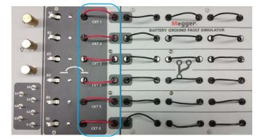
14. Once the faulted circuit is located trace the fault. This is done by moving the receiver's CT down the circuit until the fault current disappears. The point at which the fault current disappears is the location of the fault.
