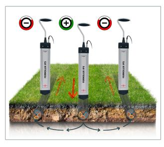
If there are several lines (cables, pipes) located next to each other, it is often difficult to determine which the correct one is. Sometimes the signal from the generator can flow through both lines, but the signal in the lines may be flowing in different directions. With the SignalSelect function, the generator applies a signal that contains directional information. When the device is positioned over the correct cable, a "+" symbol is displayed to facilitate precise identification.
