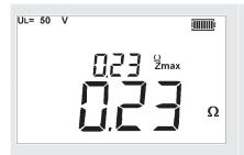
6. Move to the 2nd socket to be tested and make another loop test. If the result is less than the first the large readout will show the new value but the small readout will remain unchanged. If the new value is higher, the small readout will be updated accordingly, as below:
