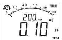
Buzzer ON = ◄)) Buzzer OFF = No symbol
