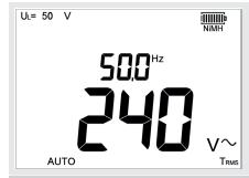
Figure 9: Instrument displaying that the circuit is live.
