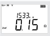
2. Switch the range knob to and make loop impedance tests as previously.
