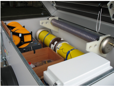
HVDC 400 integrated in trailer
